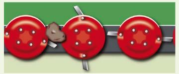
The cutterbar uses round discs that make the Profi-Line range of mowers less susceptible to stone impact.
